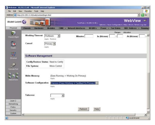
11 In the Software Configuration field, select Copy Working -> Certified on Primary for switches with a single CMM, or Copy Working -> Certified & Synchronize with Secondary for switches with a secondary CMM, then click Apply.
