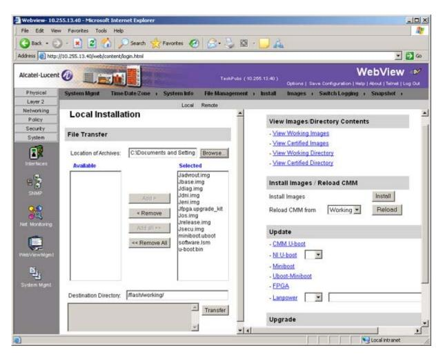
Click on the **Remove All** button to move all of the files to the "Available" area; then select the following image files and click the **Add** button to move them back to the "Selected" area as shown below: **Jadvrout.img**, **Jbase.img**, **Jeni.img**, **Jos.img**, **Jsecu.img**.
