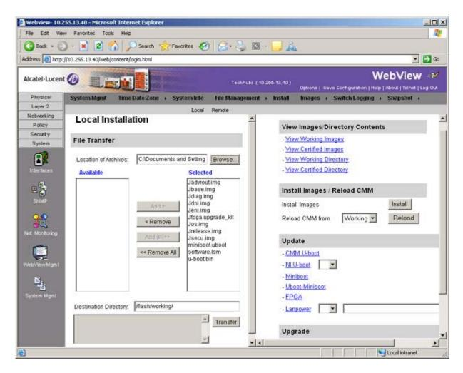
Click on the **Remove All** button to move all of the files to the "Available" area; then select both the **miniboot.uboot** and **u-boot.bin** files and click the **Add** button to move them to the "Selected" area as shown below.
